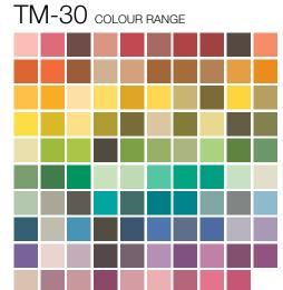
The additional information that TM30 can give is provided by two graphs that summarise the values relating to Rf, Rg and Hue Shift (a shift in the colour hue, or the perception of a false colour compared to what we would see in sunlight), and the second how the source works for groups of materials (99CES) for immediate understanding:
