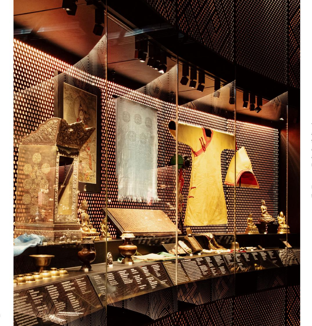
The compact size of the track and the light units combined with the high quality LED light sources and the wide variety of optics, also makes OZ suitable for use in museum environments.
